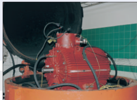
Motor ExSgm 315 M2C 260kW, 1000V, 3000 rpm tested in KD "BARBARA"
